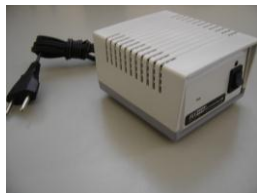
FE85C – Conversor RS232/RS422 Vista Frontal
